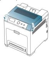
2. Open the inner cover using the handle on it.
